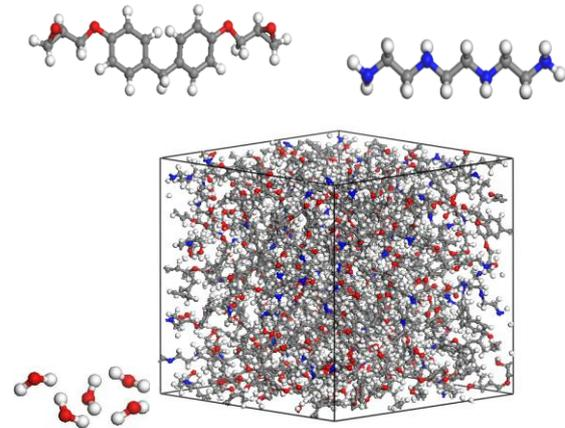
Fig. 1 Molecular model of EPON862<sup>®</sup>, TETA and amorphous epoxy
