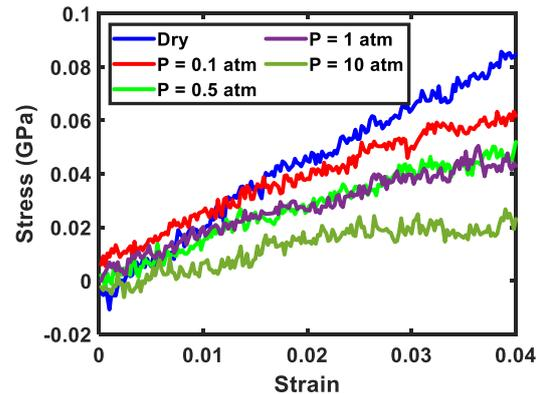
Fig. 3 Mechanical behavior of hygroscopically aged epoxy at different moisture uptake condition.
