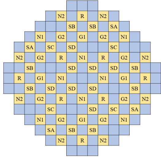
Fig. 3 Control rod configuration of CNP1000 reactor
