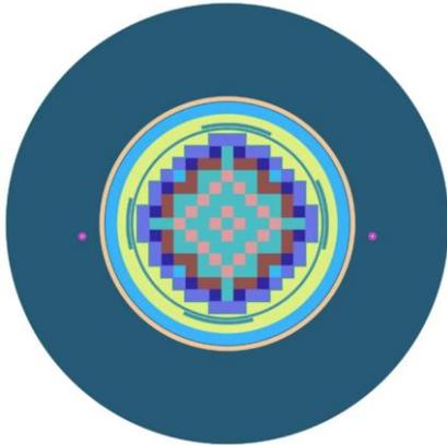
Fig. 1. Radial configuration of CNP1000 reactor
