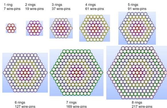
Fig. 3. Automatic wire-pin ring generation by the python program running on the SALOME GUI.
