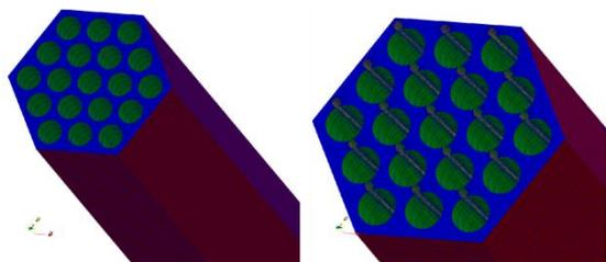
Fig. 6. A mesh for 19 wire-pin bundle generated by the programmable meshing strategy.
