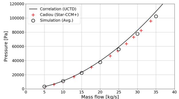
Fig. 11. Comparison of pressure drop along with mass flow for the CEA 217-pin bundle [8]
