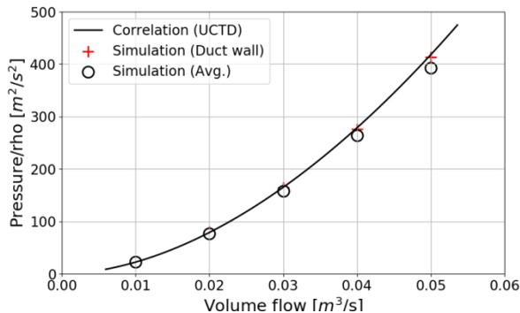
Fig. 10. Comparison of pressure drop along with volume flow for the KAERI 217-pin bundle
