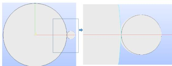
Fig. 5. Modeling of point-contact and surface-contact between a pin and a wire.
