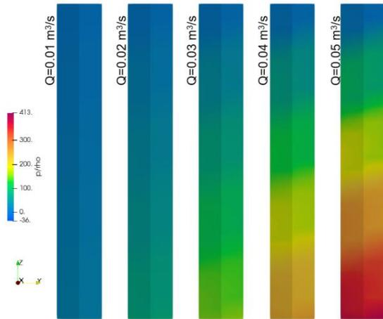
Fig. 9. Pressure distributions on the channel wall of the KAERI 217-pin bundle depending on a flow rate.
