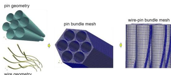
Fig. 4. Procedure of a wire-pin mesh generation
