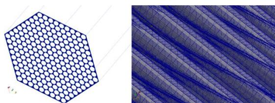
Fig. 7. A mesh for 217 wire-pin bundle generated by the programmable meshing strategy
