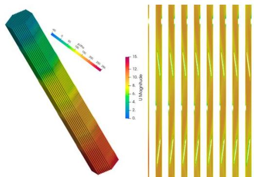
Fig. 8. Pressure and velocity distributions from the simulation of KAERI 217-pin bundle.
