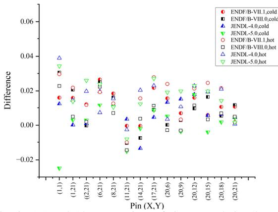
Fig. 6. KRITZ-2:13, Comparison of pin powers(C/M-1)
