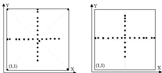
Fig. 3. Measured pin locations for KRITZ-2:13c, KRITZ-2:13h core (left) and KRITZ-2:19 (right) (Each left bottom pin position is X=1, Y=1)
