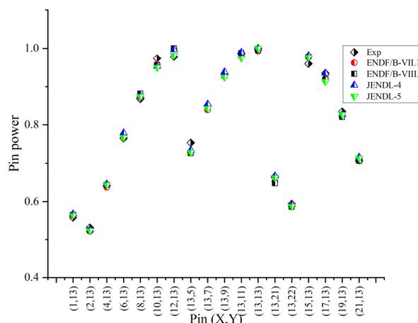
Fig. 5. Pin power distribution for KRITZ-2:19c
