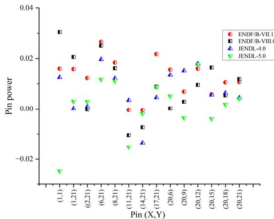
Fig. 7. KRITZ-2:19c, Comparison of pin powers(C/M-1)
