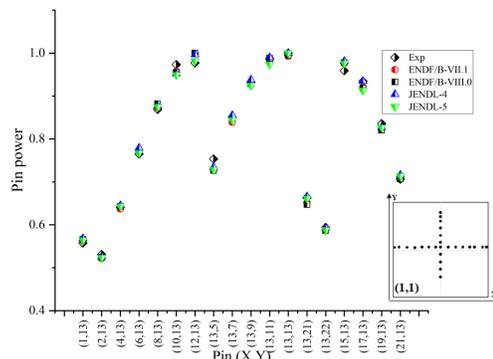
Fig.4 Pin power distribution for KRITZ-2:19c
