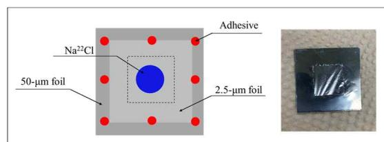
Fig 2. The positron source of  $2.5\text{-}\mu\text{m}$  Ni foil is located between the plate. We used adhesive on the side of the nickel plate.
