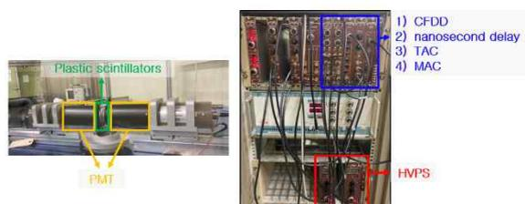
Fig 3. The NIM nodules for positron annihilation lifetime spectroscopy. PMT: photomultiplier tube HVPS: high voltage power supply, CFDD: constant fraction differential discriminator, nanosecond delay, TAC: time to amplitude converter, MCA: multi-channel analyzer.
