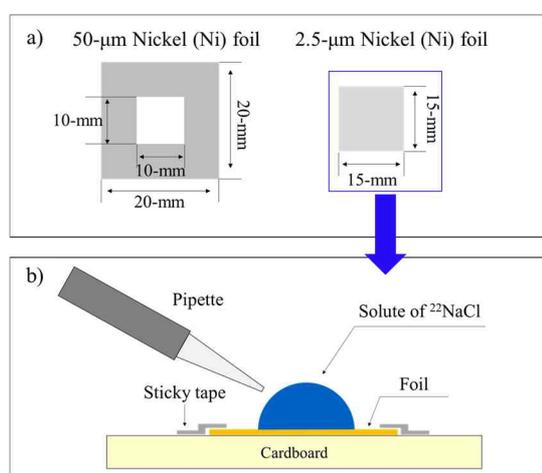
Fig 1. (a) The size of a support foil is  $15 \times 15\ \text{mm}^2$  (thickness:  $2.5\text{-}\mu\text{m}$  Ni), and the size of a disk is  $20 \times 20\ \text{mm}^2$  (thickness:  $50\text{-}\mu\text{m}$  Ni). (b) Production of positron source.
