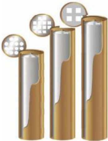
Fig. 15. Left: Canister geometries, Right: Canister overpack is made out of copper and the insert is cast iron 1)
