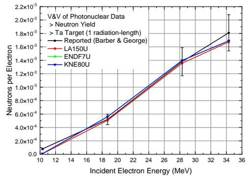
Fig. 4. Neutron yield per incident electron on a Ta target with 1 radiation-length thickness.
