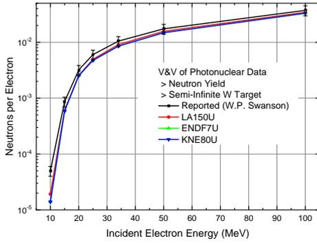
Fig. 2. Neutron yield per incident electron on a semi-infinite W target.
