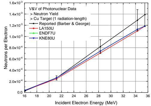
Fig. 3. Neutron yield per incident electron on a Cu target with 1 radiation-length thickness.
