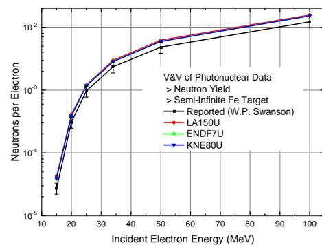
Fig. 1. Neutron yield per incident electron on a semi-infinite Fe target.
