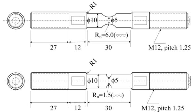
Fig. 1. Specimens used for experiment
