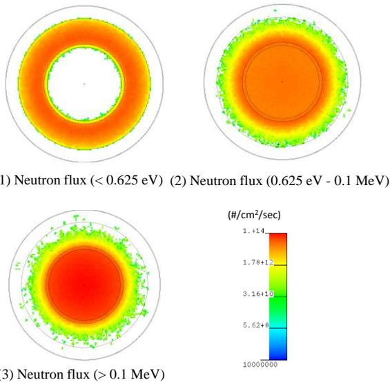
Fig. 3. Neutron flux distributions with beryllium metal outer reflector
