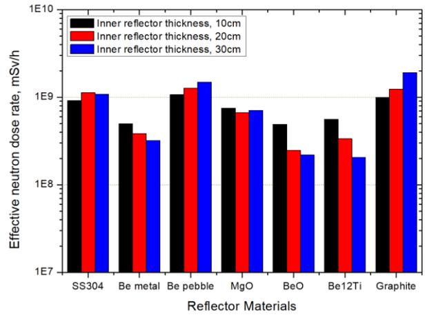
Fig. 9. Effective neutron dose rates with various inner reflector materials
