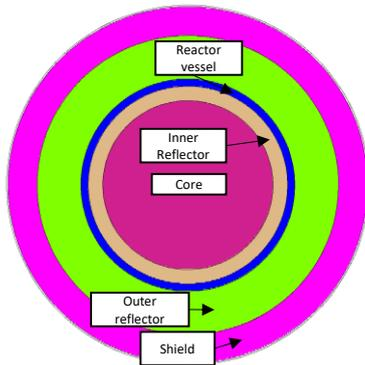
Fig. 7. An example of core model with inner reflector
