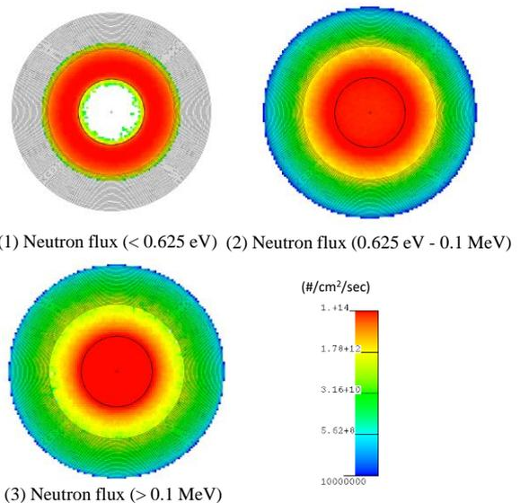
Fig. 10. Neutron flux distributions for 30 cm-thickness B<sub>4</sub>C shield case
