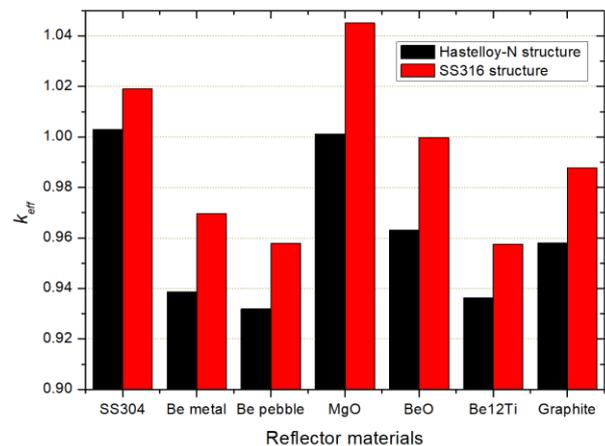
Fig. 6. Criticalities with various outer reflector materials for Hastelloy-N and SS316 reactor vessel materials
