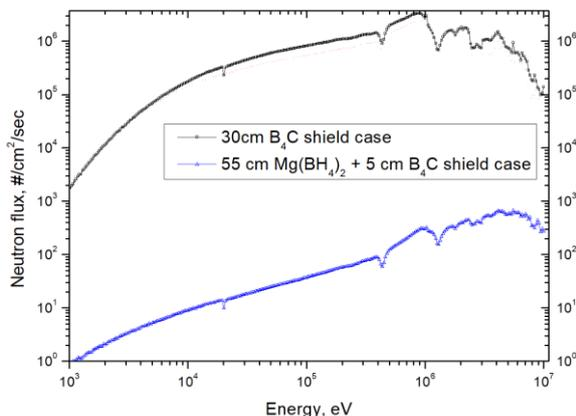
Fig. 12. Neutron spectrum of a small-size core at 1 cm distance from surface of shield
