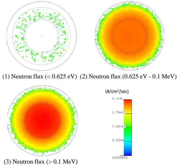
Fig. 2. Neutron flux distributions with SS304 outer reflector
