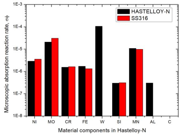
Fig. 4. Microscopic neutron absorption reaction rates
