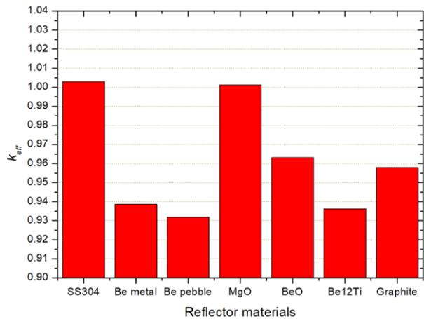
Fig. 1. Criticalities with various outer reflector materials
