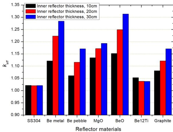
Fig. 8. Criticalities with various inner reflector materials
