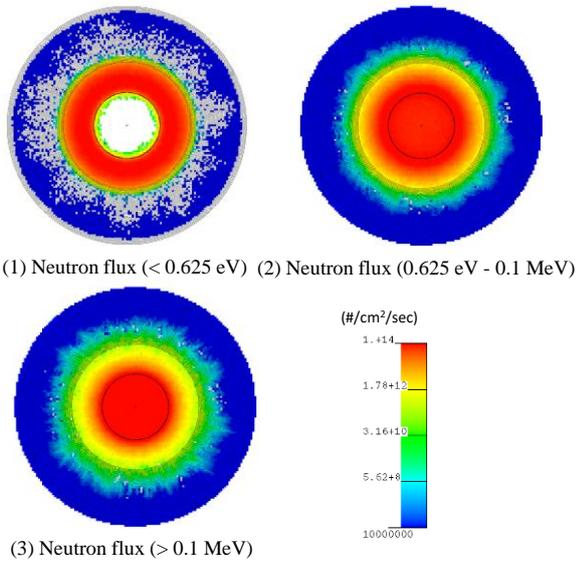
Fig. 11. Neutron flux distributions for 45 cm-thickness Mg(BH<sub>4</sub>)<sub>2</sub> and 5 cm-thickness B<sub>4</sub>C shield case
