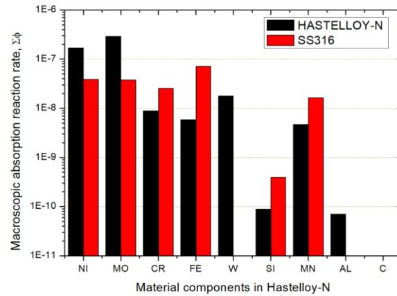
Fig. 5. Macroscopic neutron absorption reaction rates
