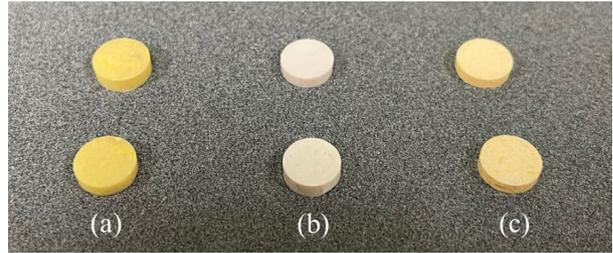
Fig. 2. Appearances of preliminary fabricated samples of control rod neutron absorber material candidates; (a)-(c) titanate group.
