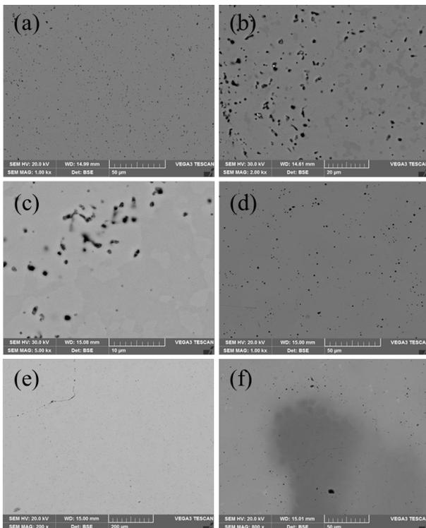
Fig. 1. Microstructure images of preliminary fabricated samples of control rod neutron absorber material candidate; (a)-(c) hafnate group and (d)-(f) zirconate group.
