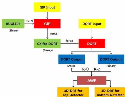
Fig. 1 The framework of DRF Generation
