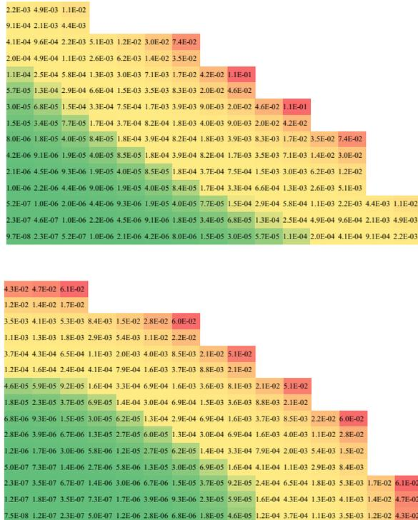
Fig. 3 Radial Distribution of DRF(Upper: Old, Lower : New)
