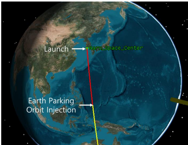
Fig. 2. Dedicated small launch vehicle trajectory from Naro Space Center (Earth Fixed Frame).
