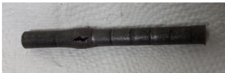
Fig. 4. Partially decladded rod-cut of 10 cm after oxidative decladding under 100% O 2 atmosphere
