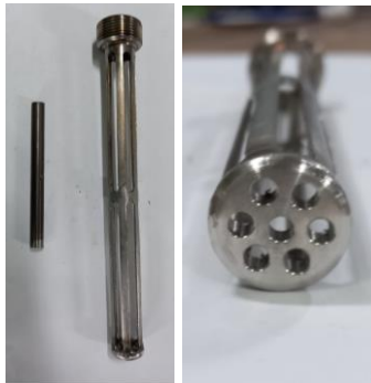
Fig. 1. Fuel basket for 10 to 20-cm rodcut
