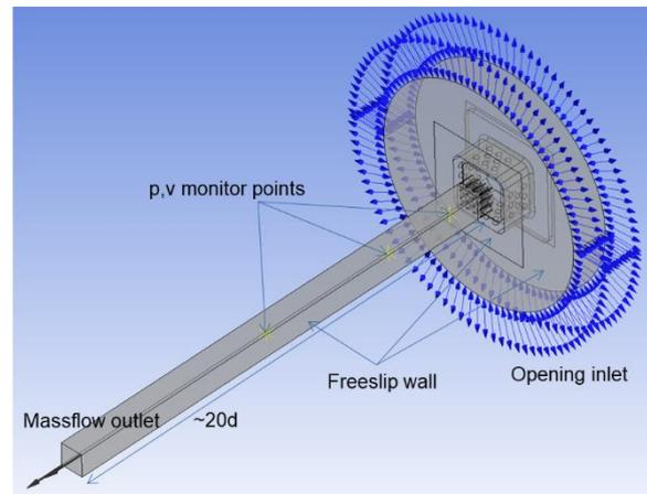
Fig. 2. Model Grid Plate Geometry
