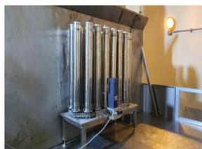
Fig. 2 To evenly irradiate the solidified waste with radiation, a separate rotating device was manufactured and worked.
