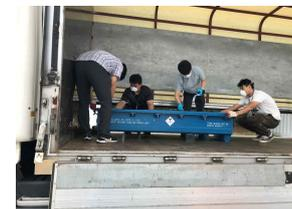
Fig. 4 Packages for transportation to transport solidified waste - unloading radioactive waste.
