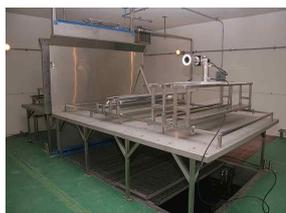
Fig. 1 High-level Gamma-ray irradiation facilities operated by the Advanced Radiation Research Institute of the Korea Atomic Energy Research Institute - 93 sources of cobalt 60 are loaded, with a total radiation dose of 193,611 Ci.
