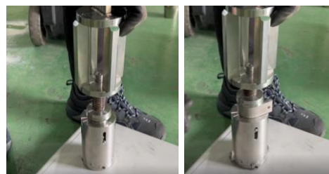
Fig. 4. Testing and the assembly of the DBD joint device
