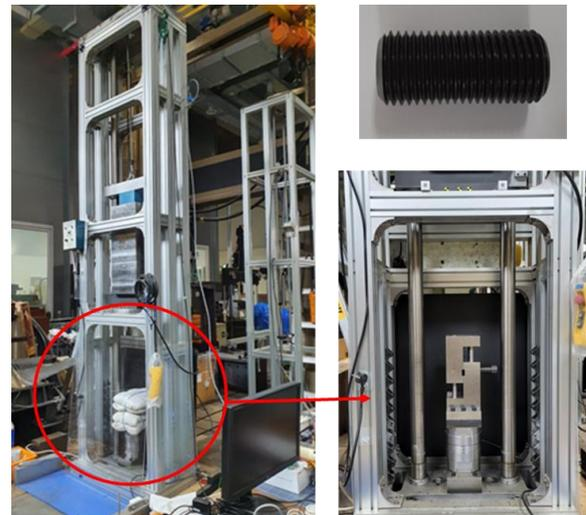
Fig. 5. Drop impact test system (Right : test specimen and jig)
