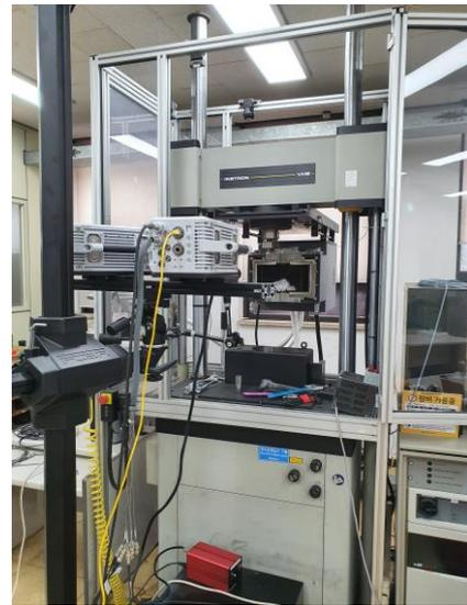
Fig. 2. High-speed tensile test facility
