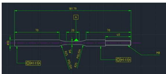
Fig. 1. High-speed tensile test specimen (mm)
