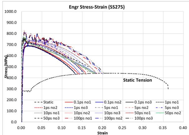
Fig. 3. Stress-strain curves of SS275 for various strain rates
