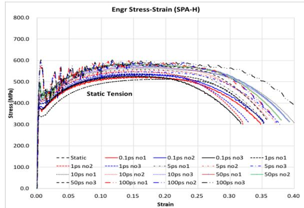
Fig. 4. Stress-strain curves of SPA-H for various strain rates
