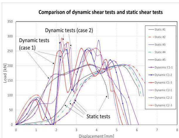
Fig. 6. Load-displacement curves of SNB7 bolt material for various drop speed
