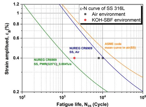
Figure 1. The EAF test results of 316L SS.
