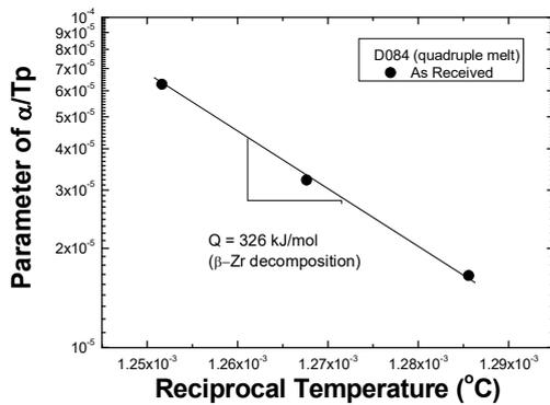
Fig. 2. Determination of activation energy for beta-Zr phase in Zr-2.5%Nb pressure tube material (quadruple melt, D084).
