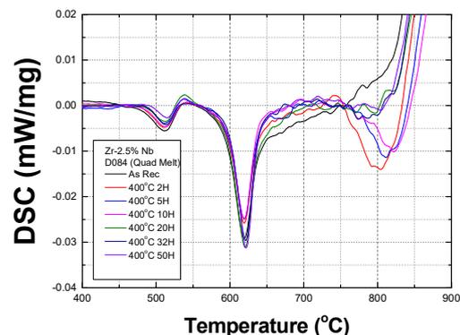
Fig. 1. DSC results of variously treated Zr-2.5%Nb pressure tube material (quadruple melt D084) aged at 400°C.
