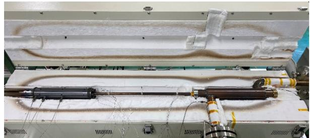
Fig. 3 Heat pipe installed inside the heating furnace
