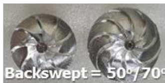
Fig. 5. Different backswept impellers for SCO 2 PE compressor
