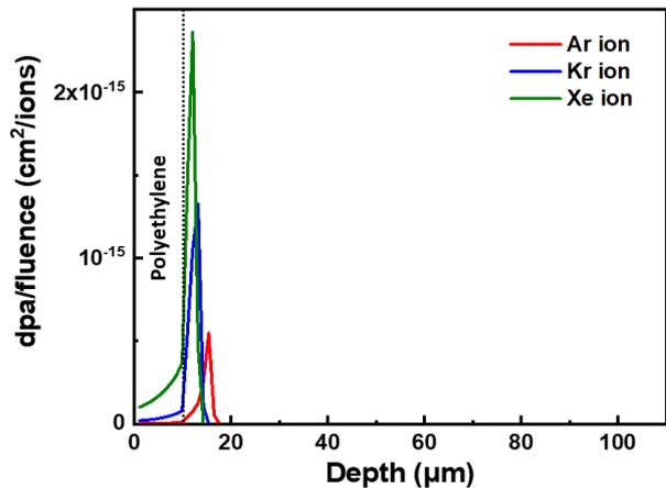
Fig. 4. Damage distribution calculated using SRIM code for tin oxyhydroxide irradiated by 50 MeV Ar, Kr, and Xe ions.
