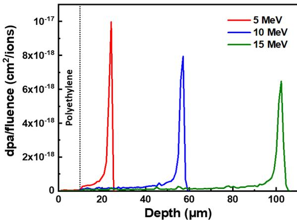
Fig. 2. Damage distribution calculated using SRIM code for tin oxyhydroxide irradiated by He ions.
