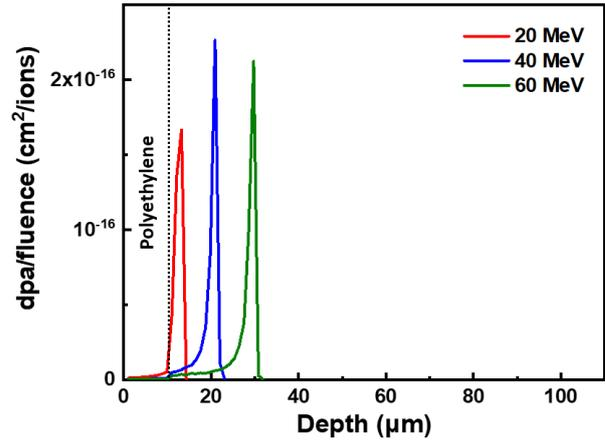
Fig. 3. Damage distribution calculated using SRIM code for tin oxyhydroxide irradiated by Ne ions.
