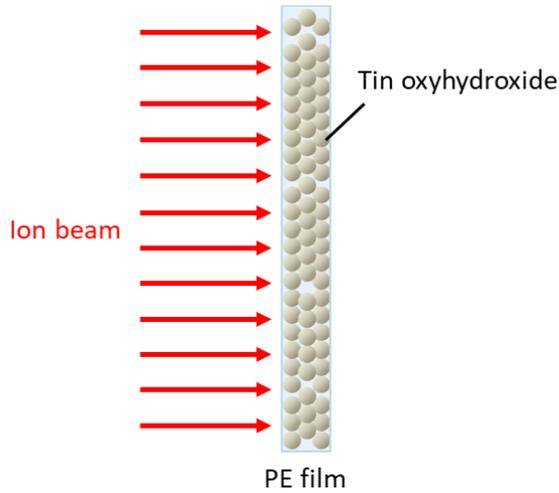
Fig. 1. Simple illustration depicting ion irradiation on tin oxyhydroxide.
