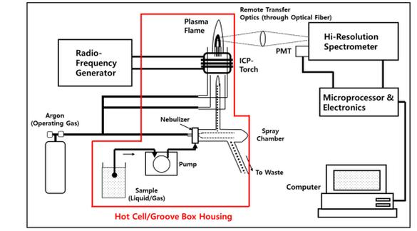
Fig. 2. Main components and typical layout of ICP-OES instrument
