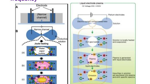
Fig. 6. Schematic principle of LEP-OES
