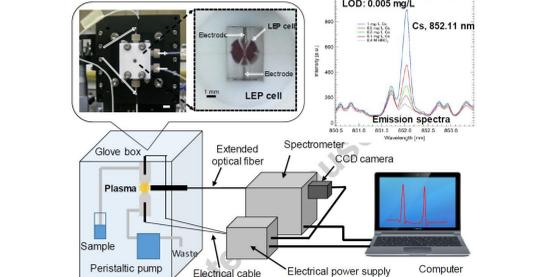
Fig. 7. Instrumentation of LEP-OES for measurement of radioactive samples
