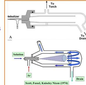
Fig. 5. Scott-double-pass Spray chamber
