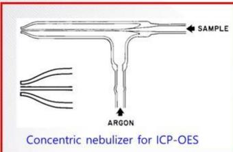
Fig. 4. The most common Nebulizer of ICP-OES
