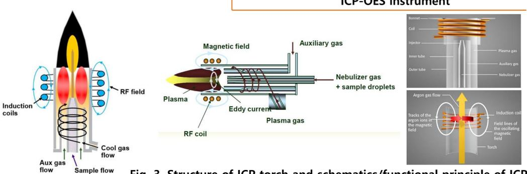
Fig. 3. Structure of ICP torch and schematics/functional principle of ICP
