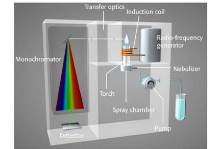
Fig. 1. Schematic structure of an ICP emission spectrometer
