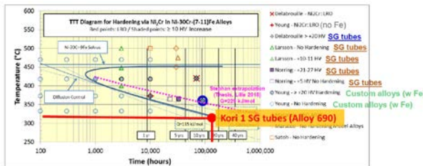
Fig. 2. Possibility of alloy 690 tubings in Kori unit 1 (Reproduced based on Ref.4)
