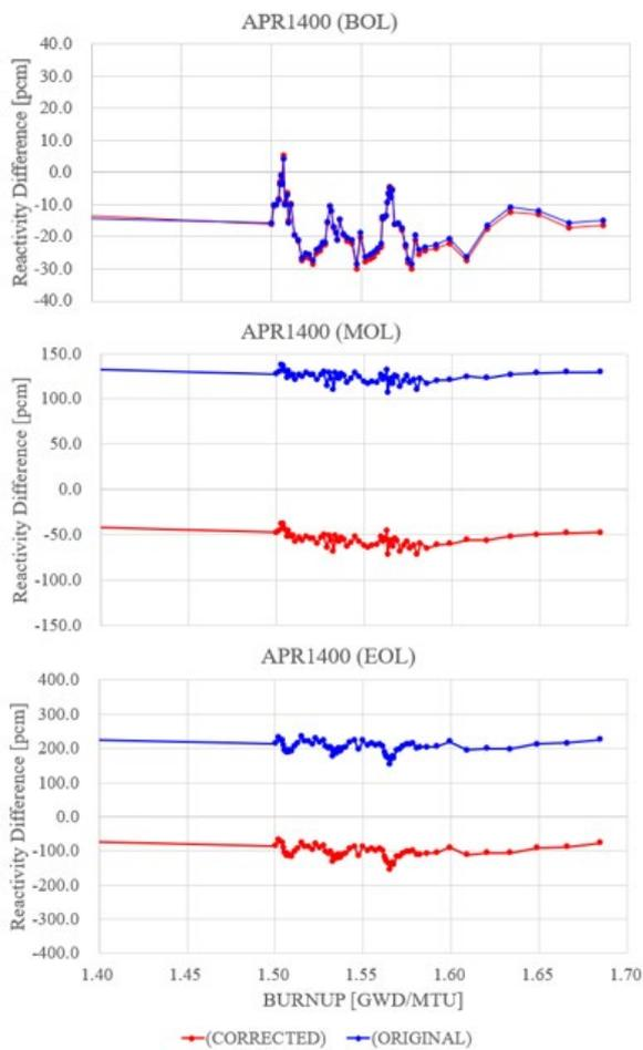
Fig. 9. Reactivity difference during LFO calculation
