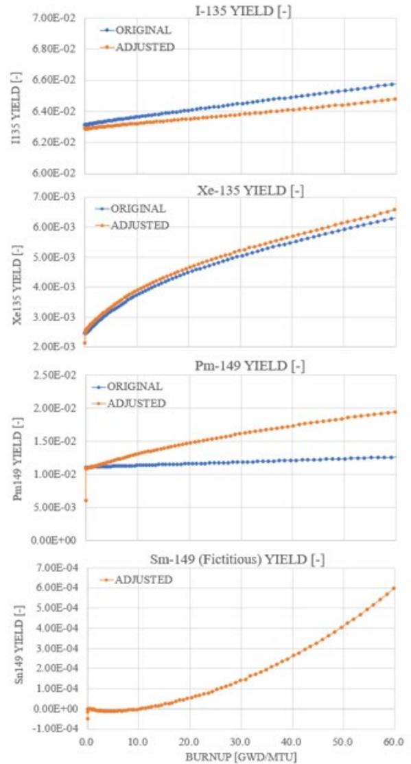
Fig. 4. Reference corrected yield values for simplified decay chains utilized in the macroscopic depletion.
