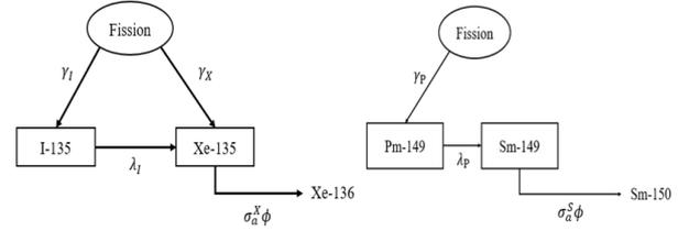
Fig. 1. Simplified decay chains for Xe-135 and Sm-149.
