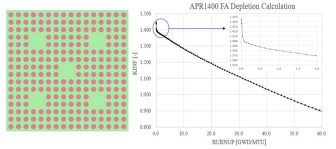
Fig. 3. Configuration of 16x16 APR1400 fuel assembly and its associated reference depletion calculation result.
