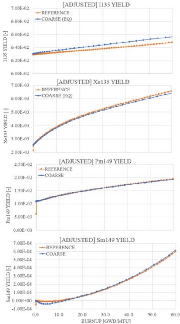
Fig. 5. Corrected fission yield values based on coarse burnup steps.
