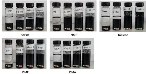
Fig. 1. Visual observation of samples 5 days after irradiation. CNT concentration 10 mg/ml, absorbed dose 0, 50, 100, and 150kGy.
