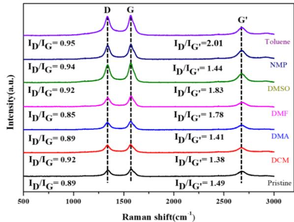
Fig. 2. Raman spectrum of CNTs after irradiation of various organic solvent dispersions.
