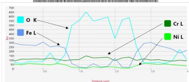
Fig. 10. The result of EDS analysis and the chromium oxide
