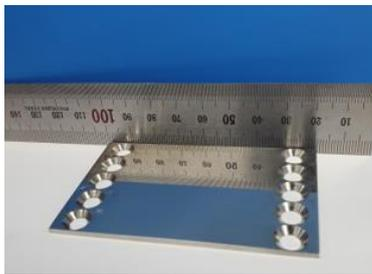
Fig. 3. The buffing-made heater and its mirror-like surface
