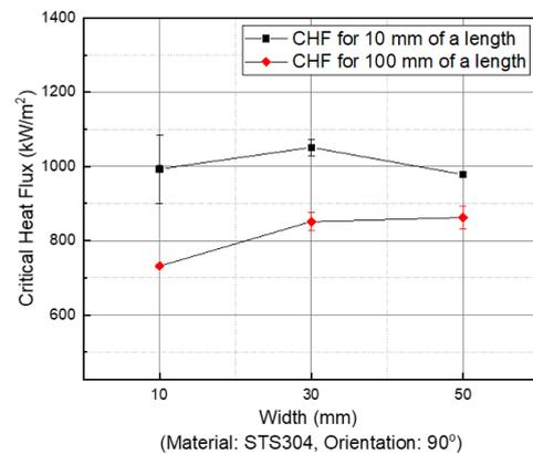
Fig. 4. The length and width effects on the CHF for the 120mesh-sandpaper-made heater
