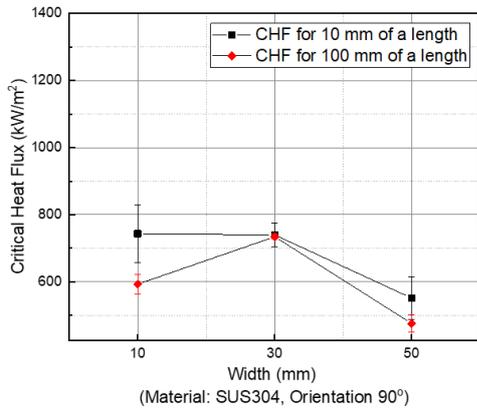
Fig. 5. The length and width effects on the CHF for the buffing-made heater
