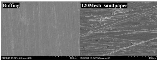
Fig. 9. The SEM image of the surface morphology made by two types of surface processes: Buffing and sandpaper
