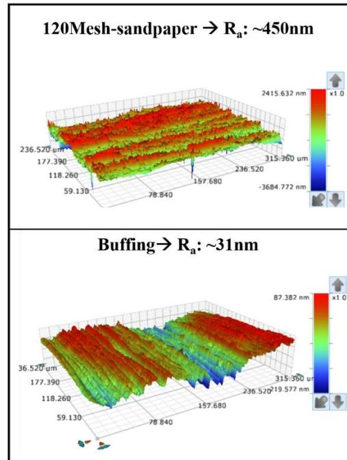
Fig. 7. The image of the 3D profile with the roughness measurement results
