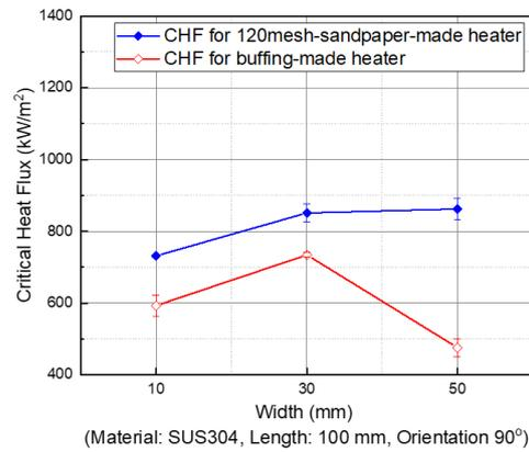
Fig. 6. The comparison of CHF values as a function of width and the surface conditions for the 100mm length heaters
