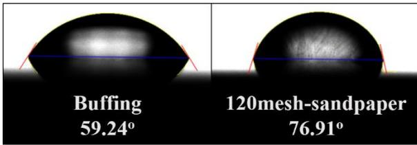
Fig. 8. The contact angle measurement depending on the surface conditions
