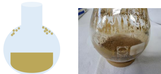
Fig. 1 Mud covered wall inside the receiving flask(left), The appearance of being Scraped soil off from the muddy wall (right)
