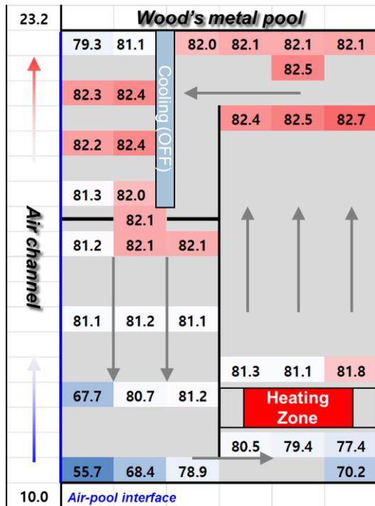
Fig. 2. Temperature distribution – 1.0 % decay heat, steady
