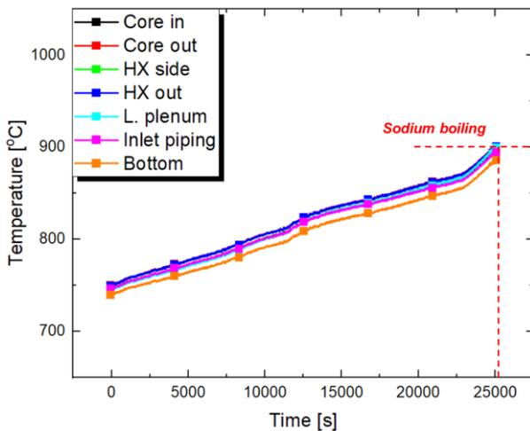
Fig. 5. Temperature behavior of the prototype, 1 → 2%
