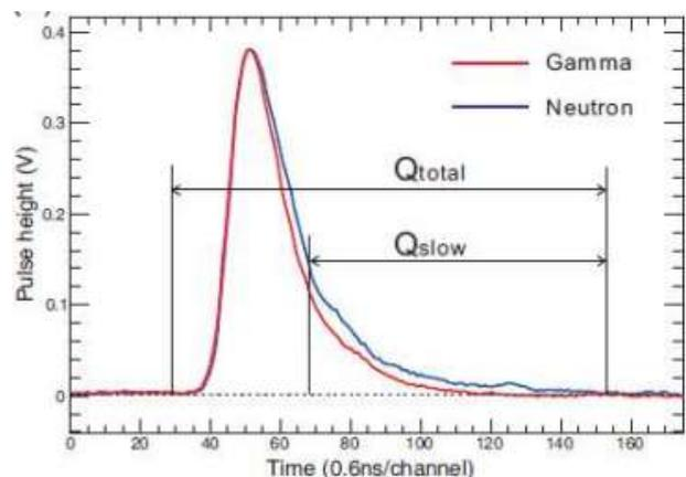
Fig 1. Typical PMT signals induced by neutrons and  $\gamma$ -rays. The  $\gamma$ -ray pulse decays more quickly than the neutron pulse, with a small difference in the tail [5].
