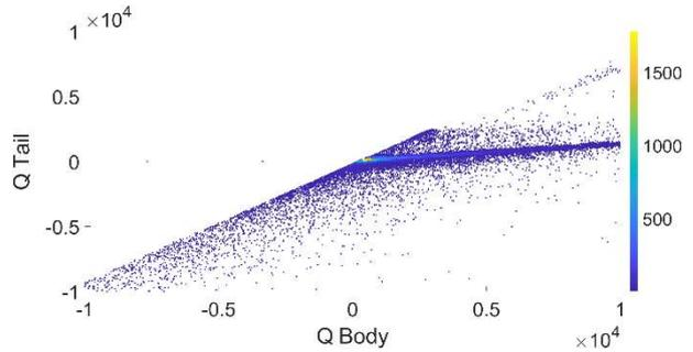
Fig. 4. PSD result based on raw pulse data collected during the 15 MeV electron accelerator operation.
