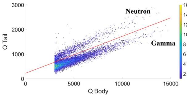
Fig. 2. The PSD result of reference  $^{252}\text{Cf}$ .
