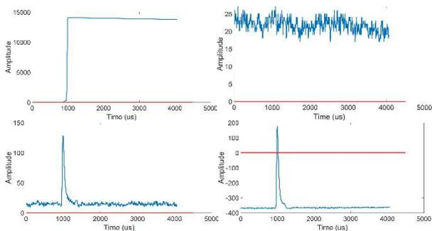
Fig. 3. Examples of pulses interrupting PSD, where red lines are desirable to be baselines. Top two pulses should be rejected and bottom two pulses should be modified with baseline correction.
