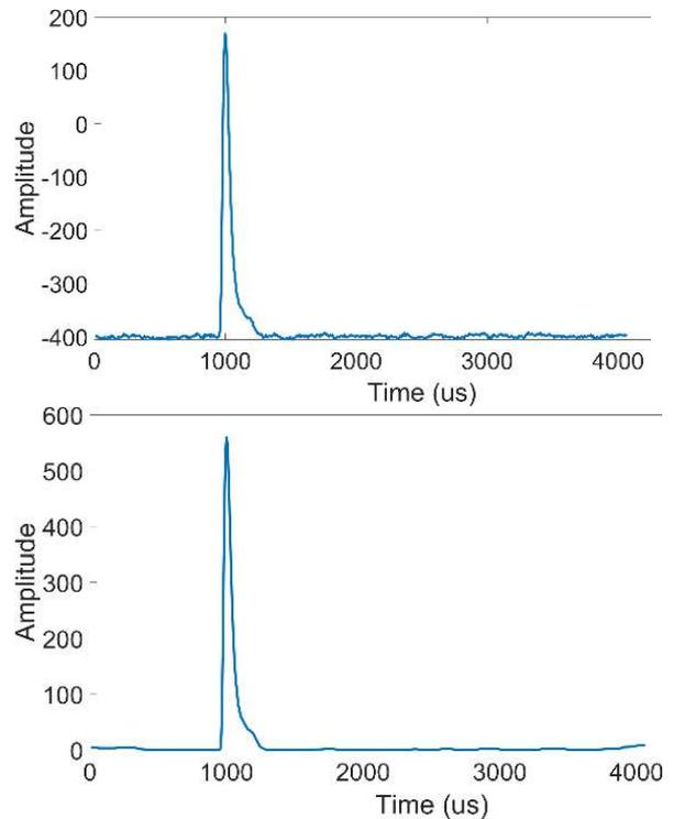
Fig. 5. Baseline shifted pulse before correction (top) and after correction (bottom)
