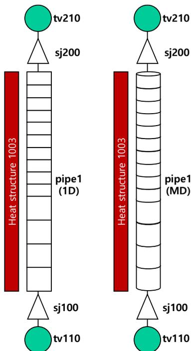
Figure 1. Schematic diagram of the modeling differences between 1D and MD
