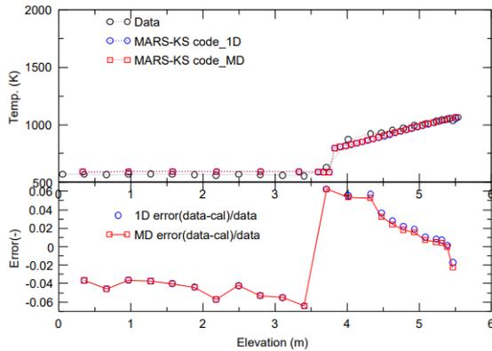
**Figure 3 QA result of Bennett test 5358
