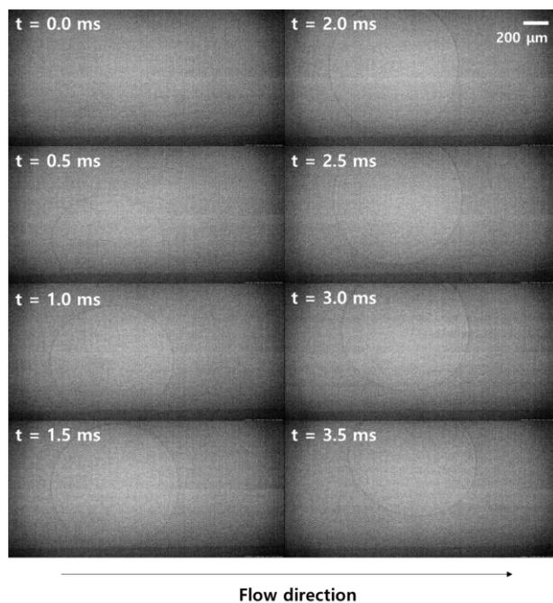
Fig. 4 Bubble growth process captured by synchrotron X-ray
