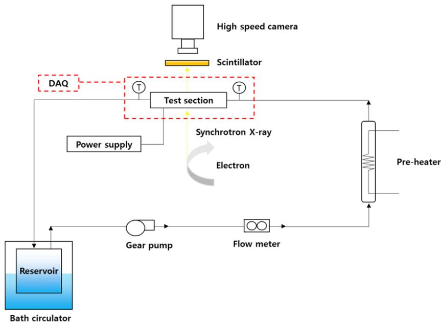
Fig. 2 Schematic of experimental flow loop.
