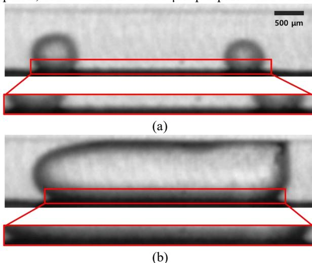
Fig. 1 High-speed camera image at flow boiling and distortion effect in  $1 \text{ mm} \times 1 \text{ mm}$  micro-channel.
