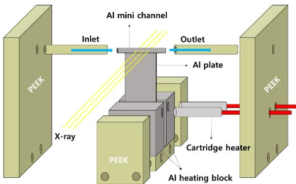
Fig. 3 Schematic of test section.
