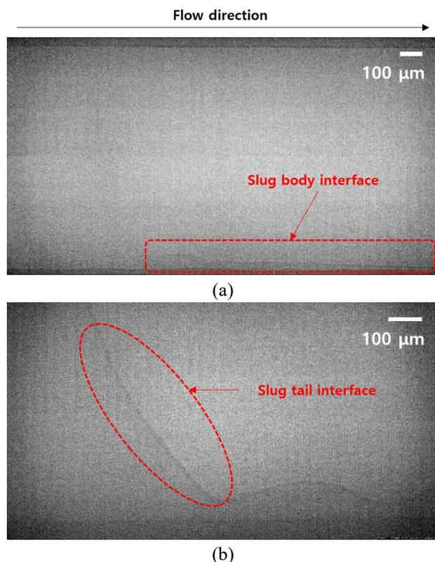
Fig. 5 Slug bubble interface image in different channel wall thickness
