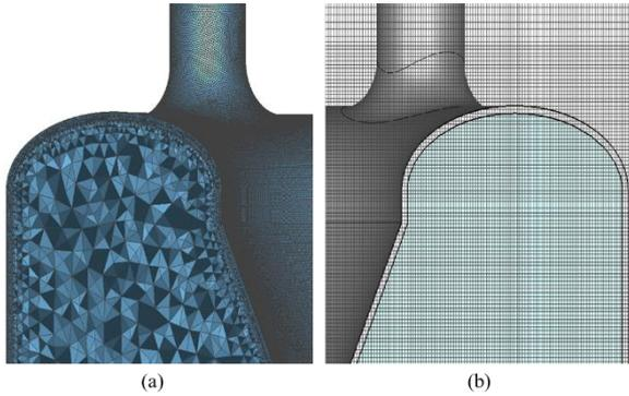
Fig. 4. (a) Tetrahedral mesh used in eigenmode solver for EM analysis and (b) hexahedral mesh used in PIC solver for MP simulation.
