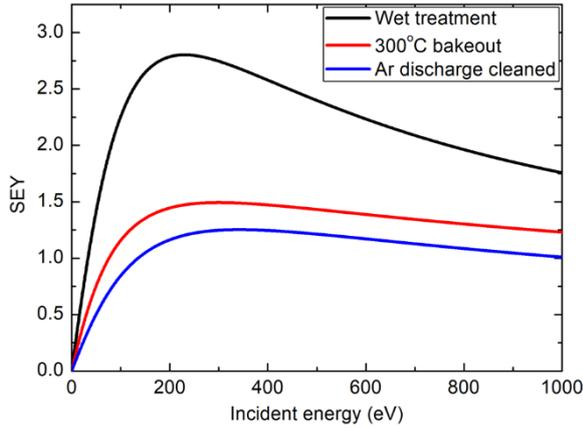
Fig. 3. Three SEY curves depending on Nb surface treatment status provided in CST PS.
