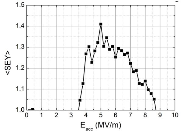
Fig. 5. Averaged secondary electron emission yield estimated by the MP simulation of the 350 MHz HWR.
