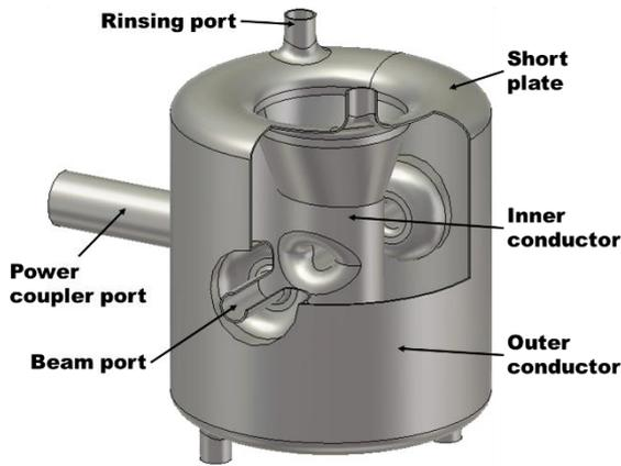
Fig. 1. Cutaway drawing of 350 MHz HWR designed for energy upgrade of the proton linac at KOMAC.
