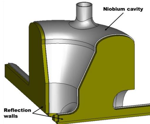
Fig. 2. 1/8 symmetric HWR cavity model and reflection walls for MP simulation.
