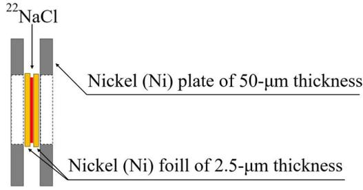
Fig 2. A structure map of a positron source
