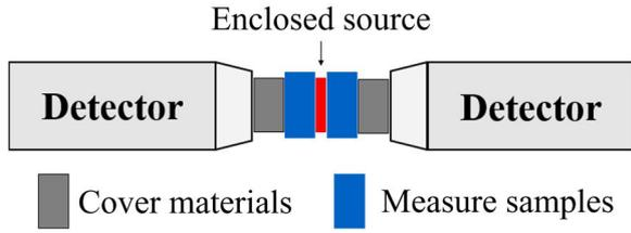
Fig 3. Structure of the detector's setting.
