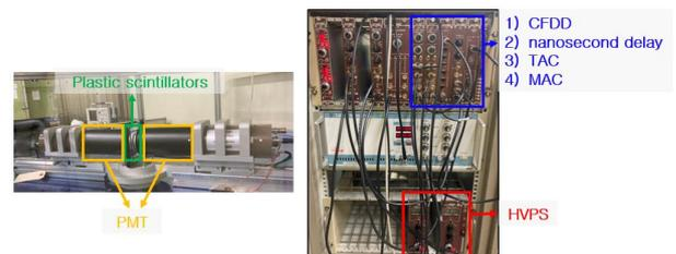
Fig 1. The NIM nodules for positron annihilation lifetime spectroscopy. PMT: photomultiplier tube HVPS: high voltage power supply, CFDD: constant fraction differential discriminator, nanosecond delay, TAC: time to amplitude converter, MCA: multi-channel analyzer.
