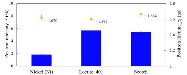
Fig 4. The blue bar is the ortho-positronium (o-Ps) intensity ( $I_3$ ) and the yellow circle is the o-Ps lifetime ( $\tau_3$ ).
