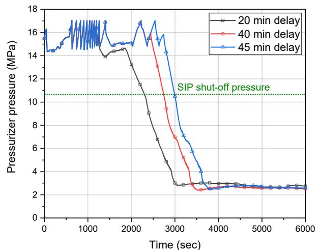
Fig. 3. Pressurizer pressure according to POSRV opening time in TLOFW
