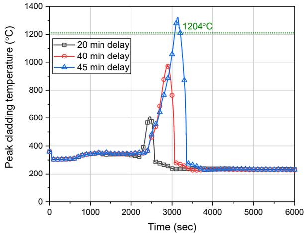
Fig. 4. Peak cladding temperature according to POSRV opening time in TLOFW
