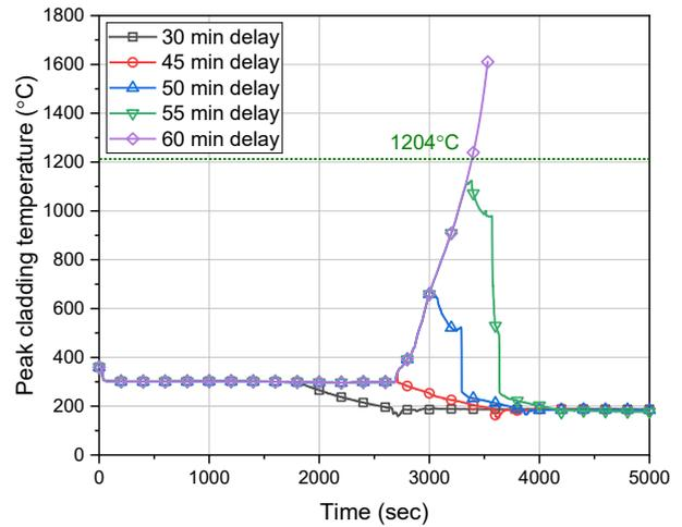
Fig. 2. Peak cladding temperature according to MSADV opening time in SBLOCA with loss of SI
