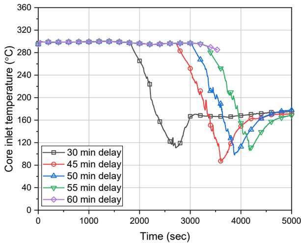
Fig. 1. Core inlet coolant temperature according to MSADV opening time in SBLOCA with loss of SI
