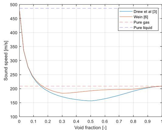
Fig. 6. Calculated two-phase sound speed of CO<sub>2</sub> at 4MPa
