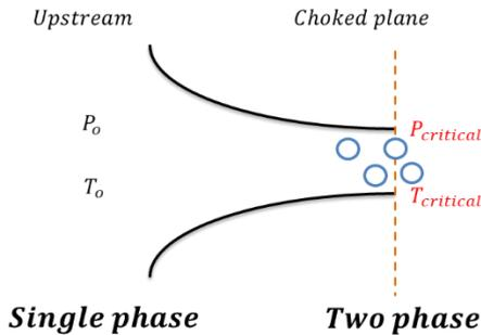
Fig. 1. Schematic of critical flow with appearance of the second phase [2]
