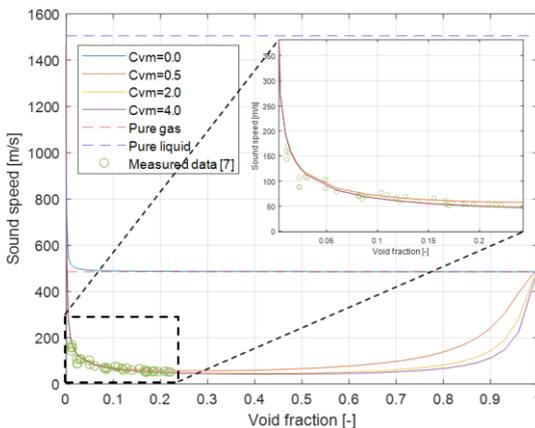
Fig. 4. Comparison of measured and calculated two-phase sound speed of saturated H<sub>2</sub>O at 265 °F
