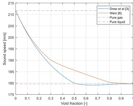
Fig. 7. Calculated two-phase sound speed of CO<sub>2</sub> at 7MPa
