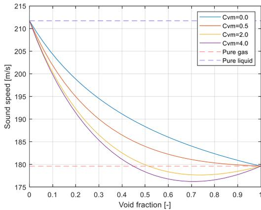
Fig. 3. Calculated two-phase sound speed of CO<sub>2</sub> at 7MPa
