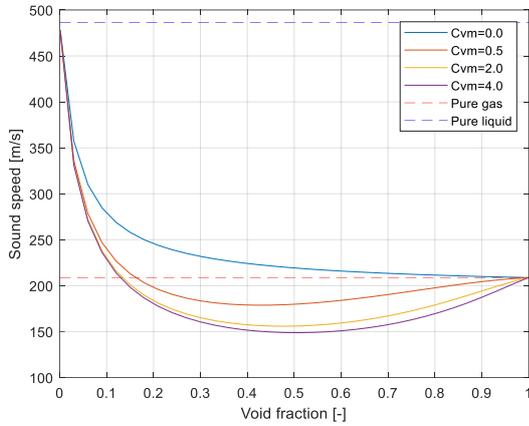
Fig. 2. Calculated two-phase sound speed of CO<sub>2</sub> at 4MPa
