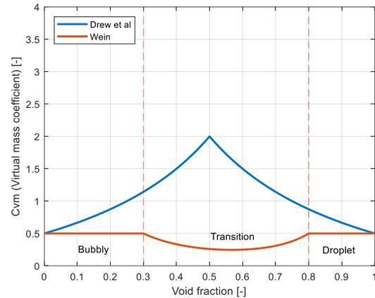
Fig. 5. Comparison of virtual mass coefficient correlations
