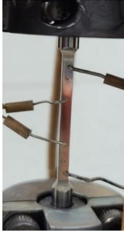
Fig. 1. Platinum probe which supplies direct current and measures potential drop
