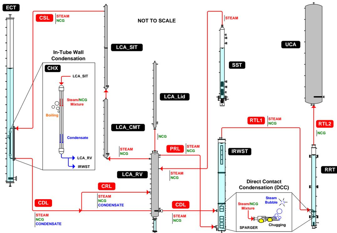
Fig. 1. Schematic diagram of SISTA2
