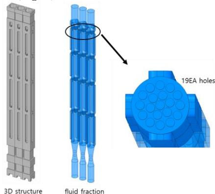
Fig. 1. Three core simulators aligned in a line and its fluid fraction for developing CFD model
