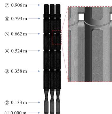
Fig. 2. Grid system of fluid fraction of the three core simulators and location at which flow rate was predicted
