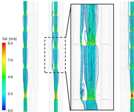
Fig. 3. Streamline flow in three aligned core simulators with APR+ operating condition and no slip wall condition
