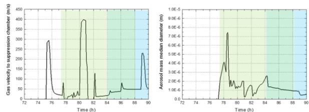
Figure 4. MELCOR results for gas velocity at the nozzle and fission product aerosol size over time.
