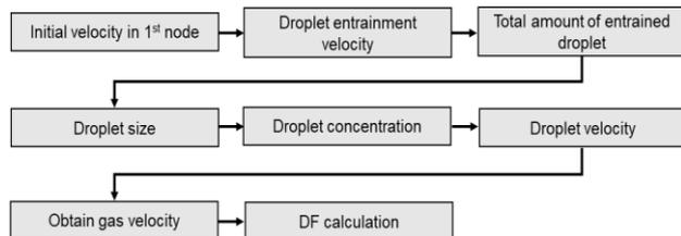
Figure 2. Decontamination factor calculation procedure in the jet pool scrubbing model.
