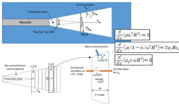
Figure 1. Schematics of the jet region to calculate aerosol removal with water droplets.
