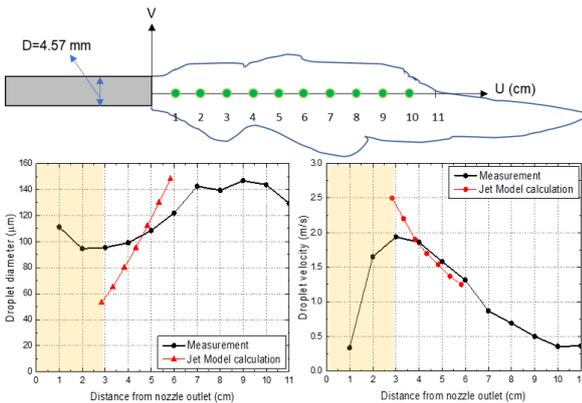
Figure 7. Droplet diameter and velocity in the jet region from PDA measurements.
