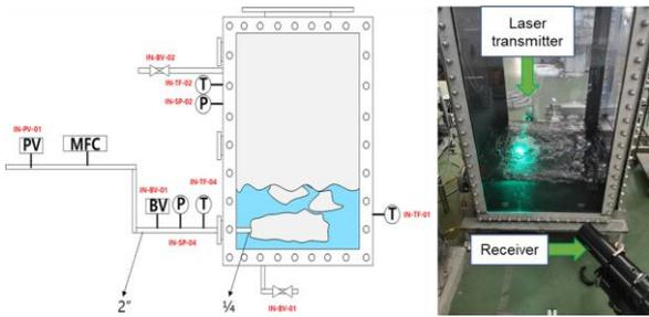
Figure 6. Experimental schematic and photograph of the PDA setup for the water droplet properties in the jet region.
