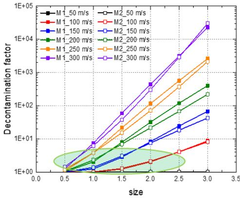
Figure 5. DF calculation during jet pool scrubbing in FK2.
