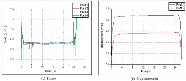
Fig. 3. Strain and displacement of T4 transport package
