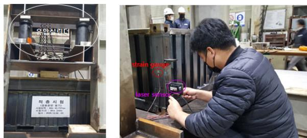
Fig. 2. Stacking test of T6 transport package
