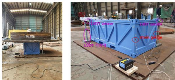
Fig. 1. Stacking test of T4 transport package
