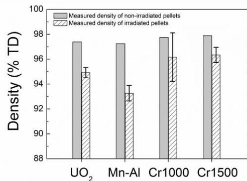
Fig. 4. Porosity and pellet density changes after the resintering and irradiation.
