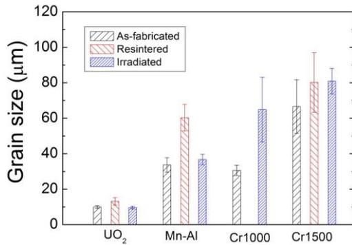
Fig. 5. Averaged grain size change of the samples after the resintering and irradiation.
