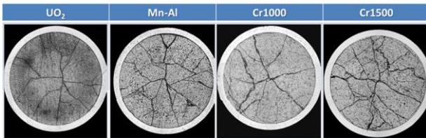
Fig. 2. Cross sectional optical micrographs of irradiated sample pellets
