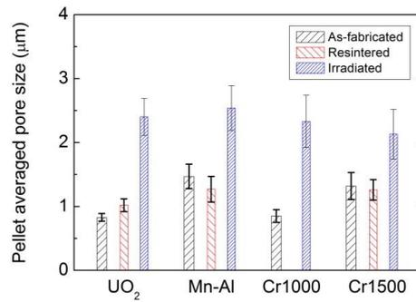
Fig. 3. Pore density and pore size changes after the resintering and irradiation.
