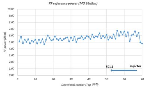
Fig. 8. Power level for LLRFs and BPMs on each tap of the RF reference line
