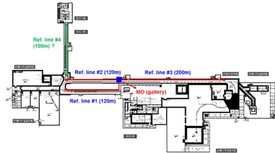
Fig. 1. Schematic layout of the RF reference lines and the reference-feed in the linac tunnel
