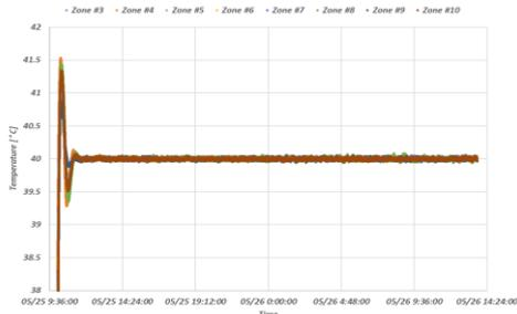
Fig. 4. Temperature control results on the RF reference line (Test results:  $< 40 \pm 0.1$  °C)
