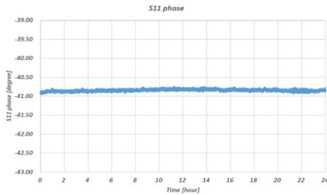
Fig. 5 phase stability on the RF reference line ( $< \pm 0.1$  °)
