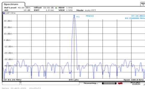
Fig. 7. Power level of the master oscillator
