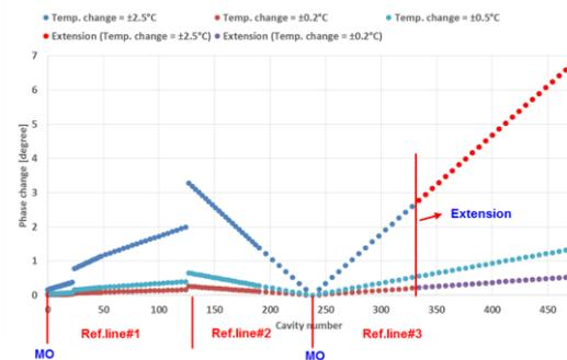
Fig. 2. Phase change ("degree" corresponds to the cavity RF frequency) due to temperature change for each of the cavity along the linac.
