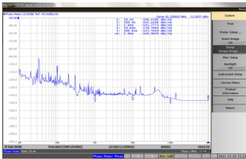
Fig. 6. Measured phase noise of the 81.25 MHz reference (Calculated jitter: 588fs, Calculated phase error:  $0.0172^\circ$ )
