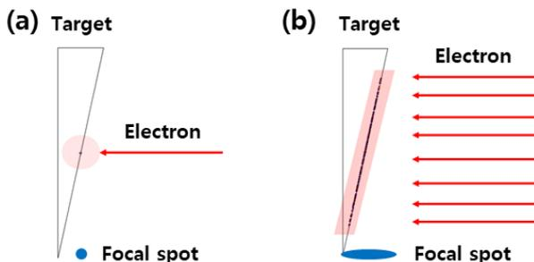
Fig. 3. Focal spot of X-rays at the (a) lowest tube current and (b) highest tube current.
