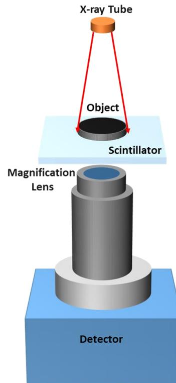
Fig. 1. Illustration of a general X-ray imaging system.
