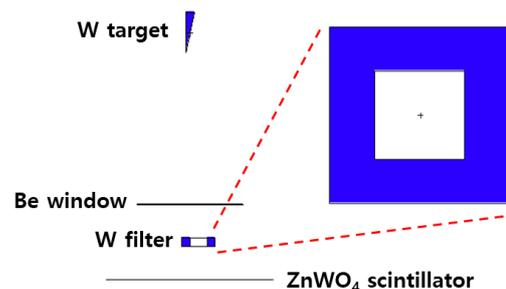
Fig. 2. Simple description of the X-ray scintillation part for MCNP dose simulation.
