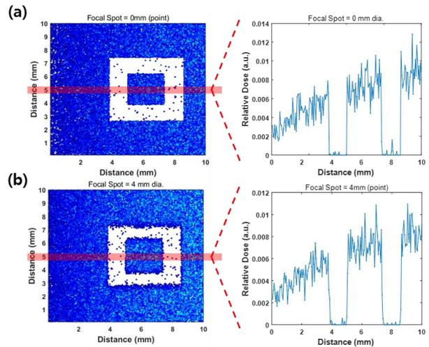
Fig. 4. Absorbed dose distribution of ZnWO<sub>4</sub> scintillator and relative dose corresponding to the red line by X-rays with a focal spot of (a) zero and (b) 4 mm.
