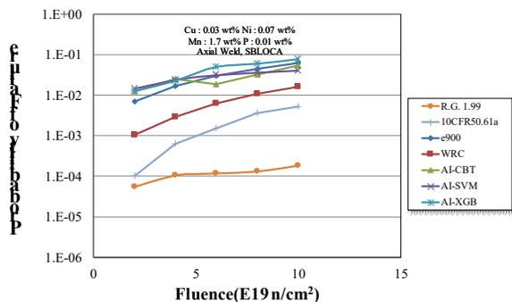
Fig. 3. Comparison of failure probability (SBLOCA)
