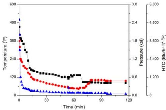
Fig. 2. Time dependent temperature, pressure and film coefficient profile (SBLOCA)
