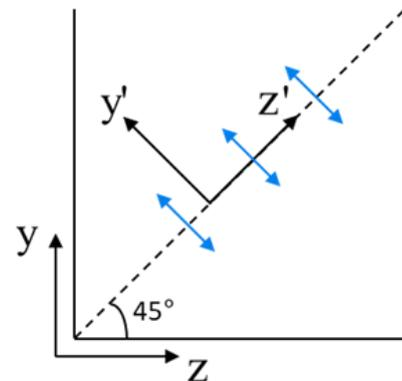
Fig. 5. Line of symmetry between two perpendicular walls with different coordinate systems
