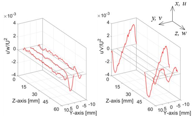
Fig. 3. Normalized Reynolds shear stresses for  $u'w'/U^2$  and  $u'v'/U^2$  in the forced convection condition ( $Re_{in} = 5500$ ,  $T_{out} - T_{in} = 32.7K$ )
