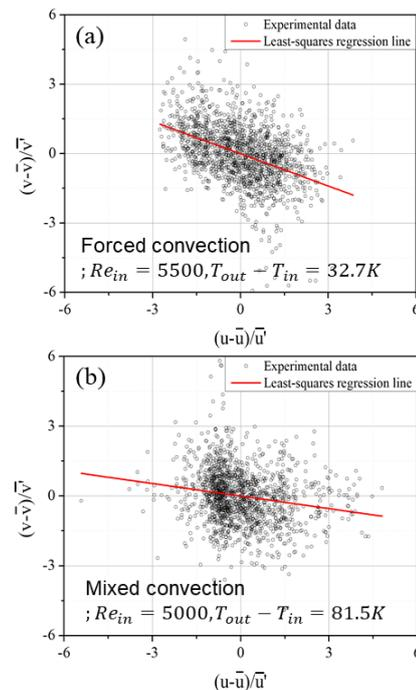
Fig. 1. Quadrant analysis results in the forced convection (a) and mixed convection (b) conditions.
