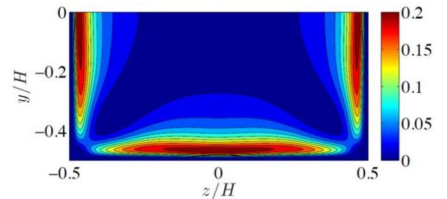
Fig. 4. DNS analysis result for the production of turbulence kinetic energy scaled with  $u_{\tau,c}^4/\nu$  inside a square duct ( $Re_{\tau,c} \approx 180$ , Marin et al., 2016)
