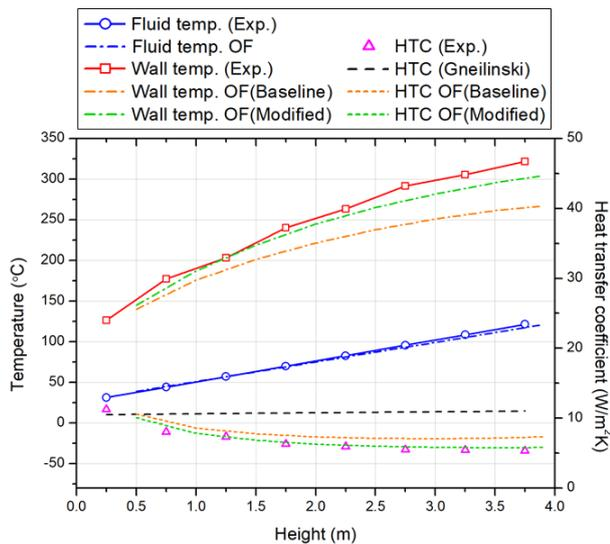
Fig. 6. Experimental data and CFD analysis results with and without the modification of the turbulence model (RHEF experiment,  $Re_{in} = 8921$ , heat flux =  $1070 \text{ W/m}^2$ ).
