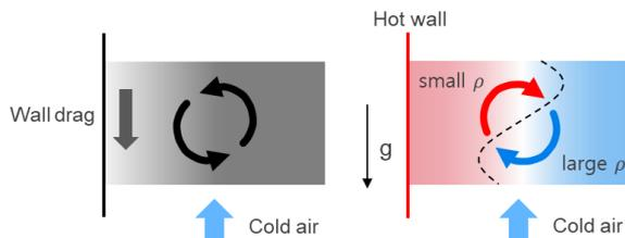
Fig. 2. Formation of wall-bounded and horizontal density ( $\rho$ ) gradient-induced vortices near the heated wall.
