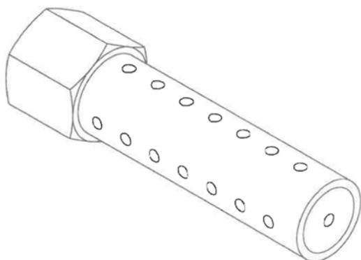
Fig. 5 Multi-hole nozzle used for tests.
