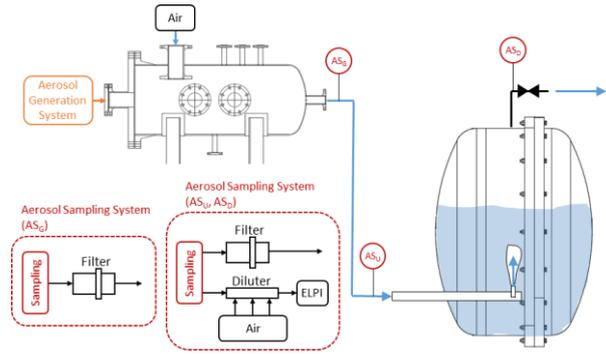
Fig. 4 Scaled-down test facility of the suppression tank
