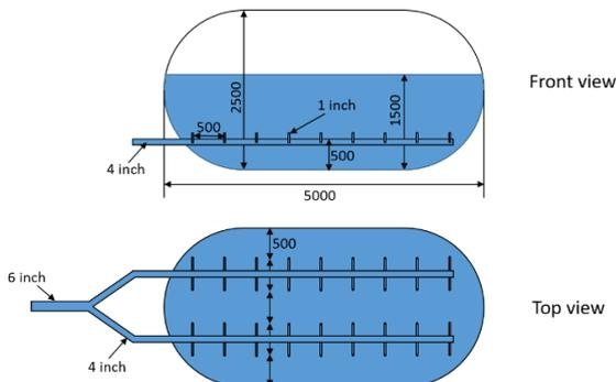
Fig. 3 Suppression tank of bypass accident mitigation system
