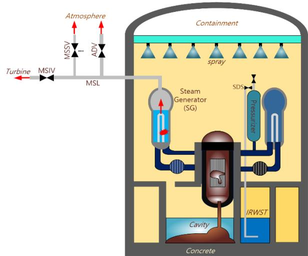
Fig. 1 Schematic of Bypass Accident by SGTR
