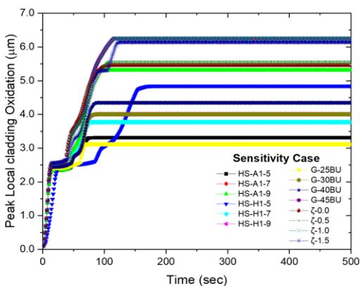
Fig. 9. Peak local cladding oxidation
