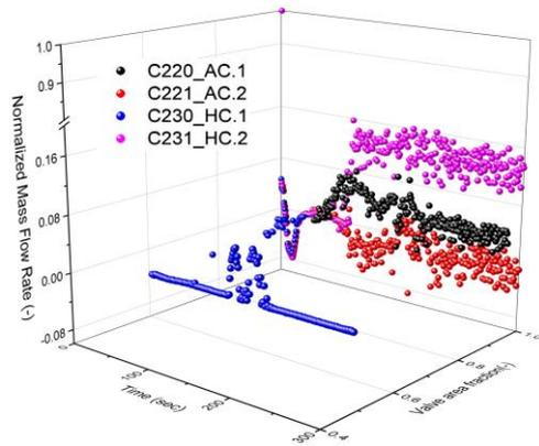
Fig. 4. Flow rate according to core flow area change
