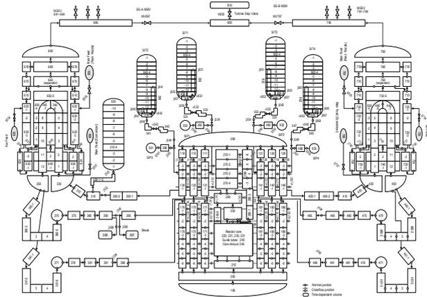
Fig. 1. MARS-KS nodalization for LBLOCA of APR1400
