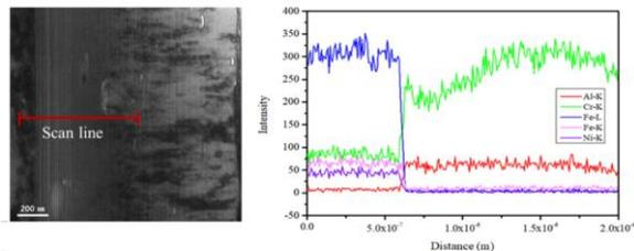
Fig 3. Cross-sectional TEM image and line scan mappings of CrAl coated specimen
