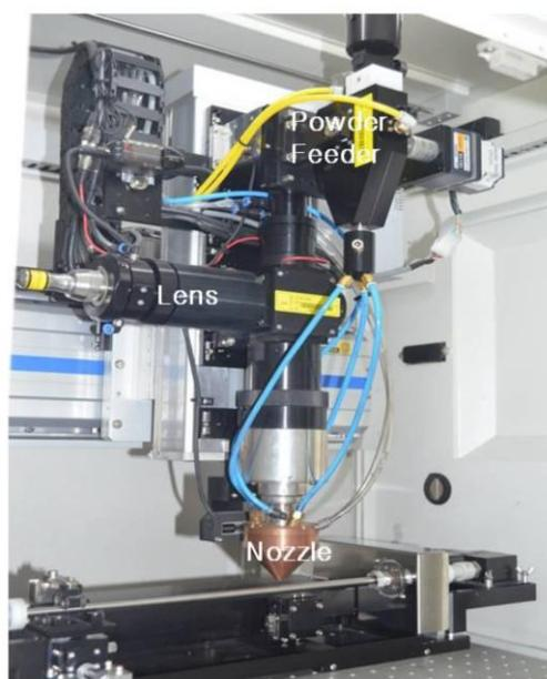
Fig 1. Appearance of the laser equipment for coating (adapted with permission from ref. [1].
