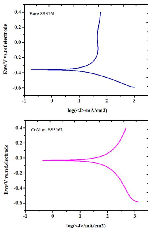
Fig . Polarization curves of bare SS316L and CrAl coated SS316L in 0.5 M H<sub>2</sub>SO<sub>4</sub> solution at 80 °C
