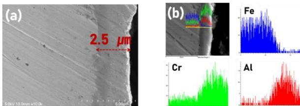
Fig 2. (a), (b) show the cross-sectional SEM-EDS analysis of the CrAl coating layer.
